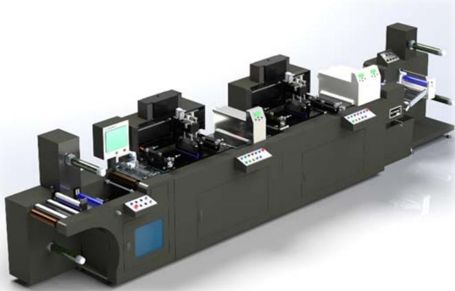
Full servo printing unit control system, printing speed and ink return speed freely adjustable
